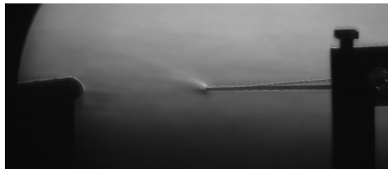
Figure 1: Preliminary schlieren imaging of a corona discharge
